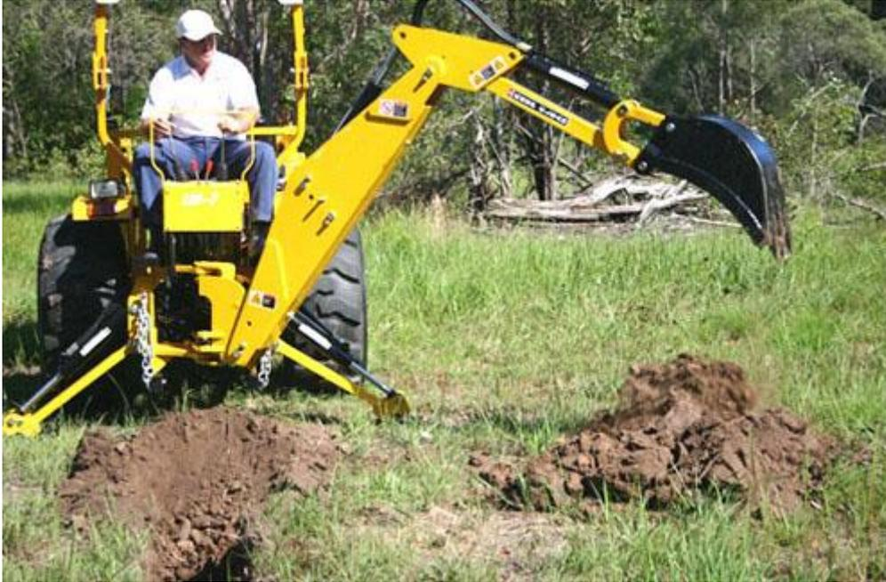
The LW series backhoe is a strong design, it is used for ditching in farms and grazing lands, digging pool, cleaning water ways as well as assistant excavating work in construction and building roads.
