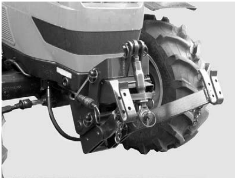
Front three point linkage
